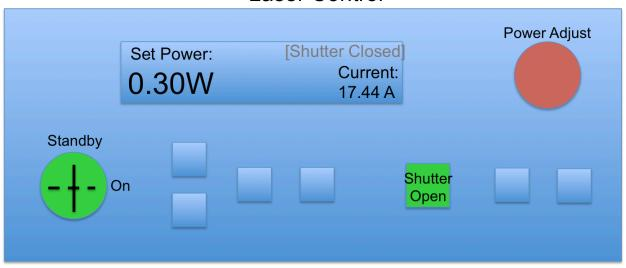
Schematic: Items in GREEN require attention before operating experiment; item in RED must remain AS-IS; do not adjust. When shutter is open, grey "shutter closed" indication does not appear.
